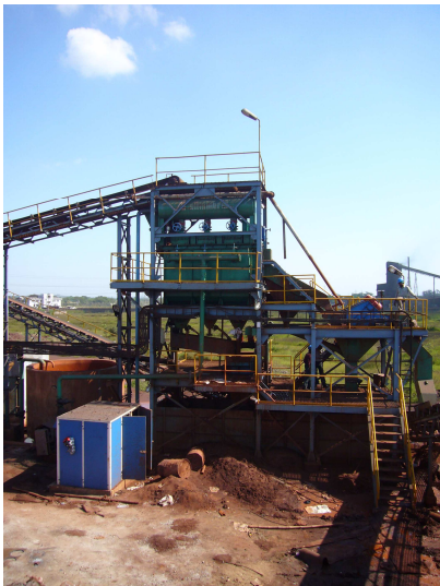
Fig. 5: Low grade lump ore jig at OCL jig plant, India
