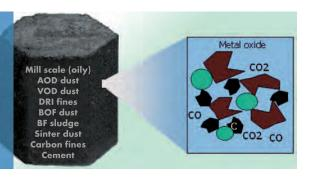
In contrast to other alternative iron making processes the OXYCUP® melt shop directly produces liquid hot metal similar to blast furnace quality. A C-Brick may be composed of a variety of different ingredients. In particular matter with high iron content like BOF dust or sludge is welcome, but also matter with high carbon content like BF sludge. The agglomerates are produced on site in the C-Brick agglomeration plant.
